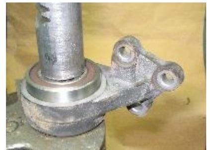
9. take off the bearing and used seals from the bracket body.
