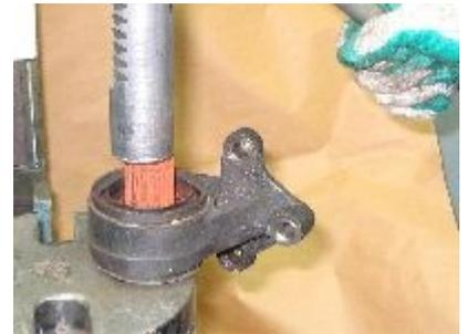
7. Slide off the joint from the axle using a hammer.
